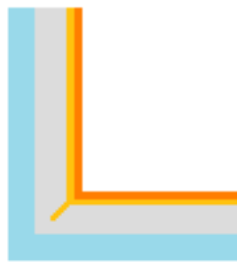
Internal treatment against negative water pressure using a chase.
