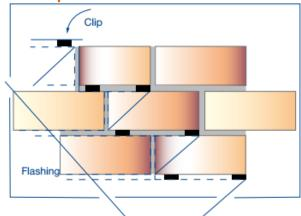
2. Completed installation of the clip into the standard brick joint.
