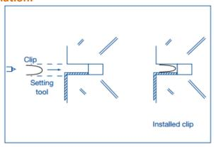
1. Insertion of the clip by means of the setting tool.
